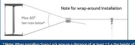
\* Note: When installing Span-Lock ensure a distance of at least 1.5 × the height of the beam is left between the Zip-Clip locking device and the structure. An installation angle of 60° should not be exceeded.
